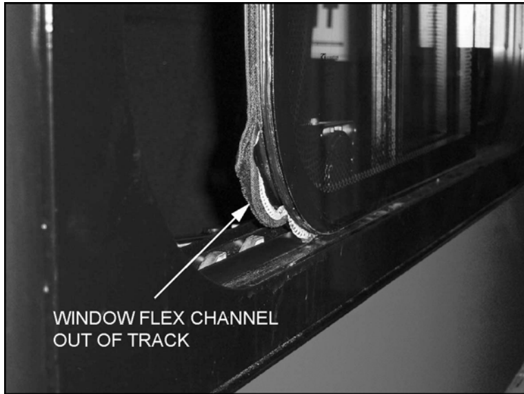
Figure 1: Window Flex Channel "Schlegel" (Out of Track)
