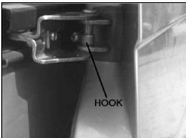
FIGURE [8]: REAR HOOK INSTALLED
