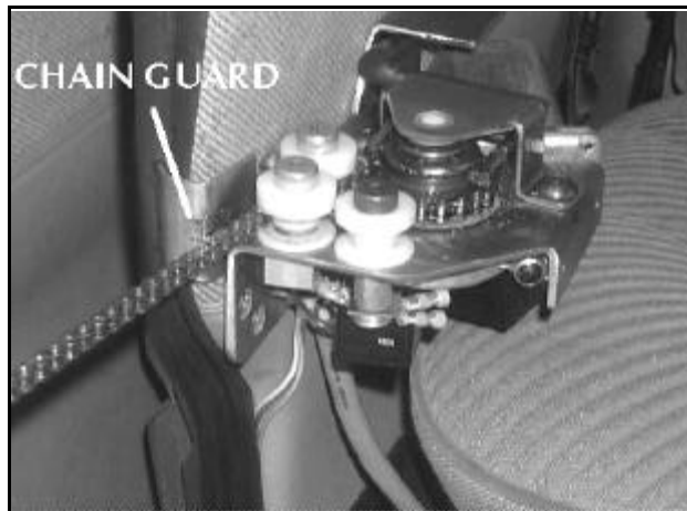
FIGURE [5]: CHAIN GUARD AND D.O. INSTALLED
