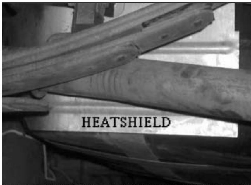
**FIGURE [2]: HEATSHIELD REMOVAL**
