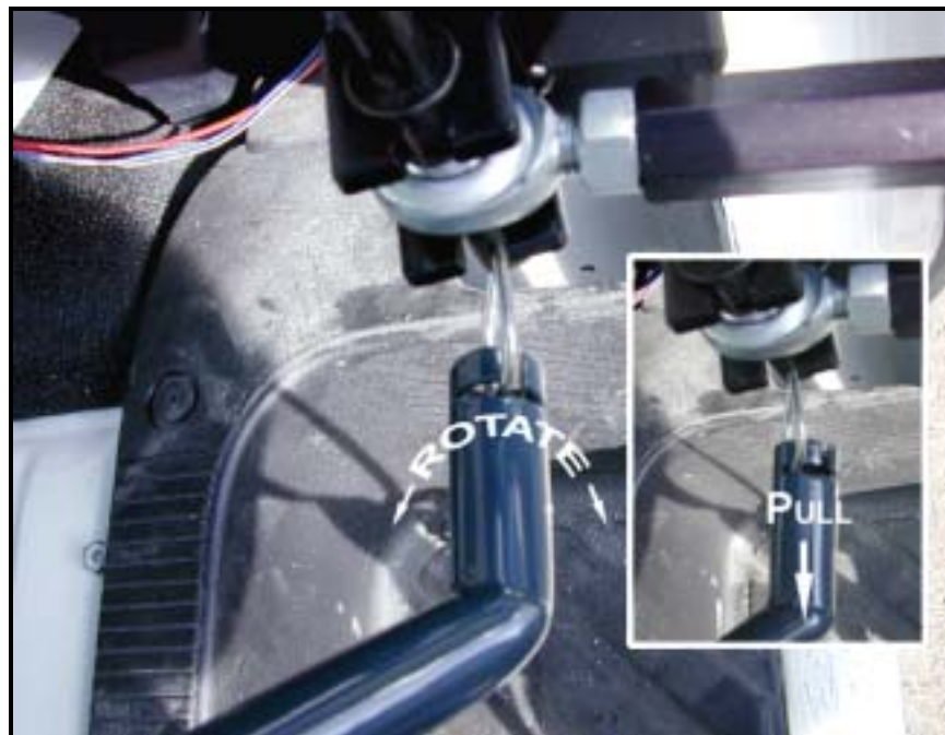
Figure [35] HITCH PIN REMOVAL
