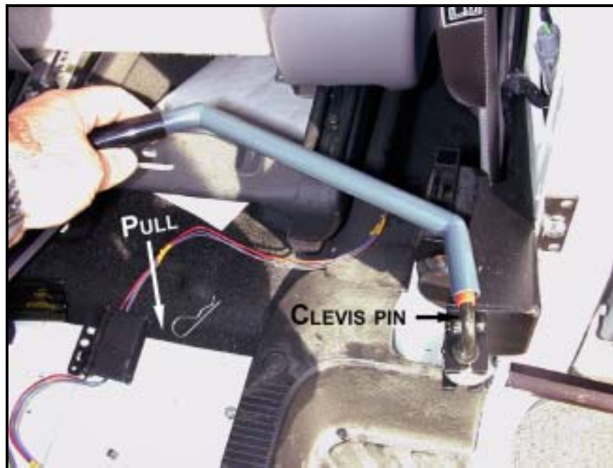
Figure [36] CLEVIS PIN REMOVAL
