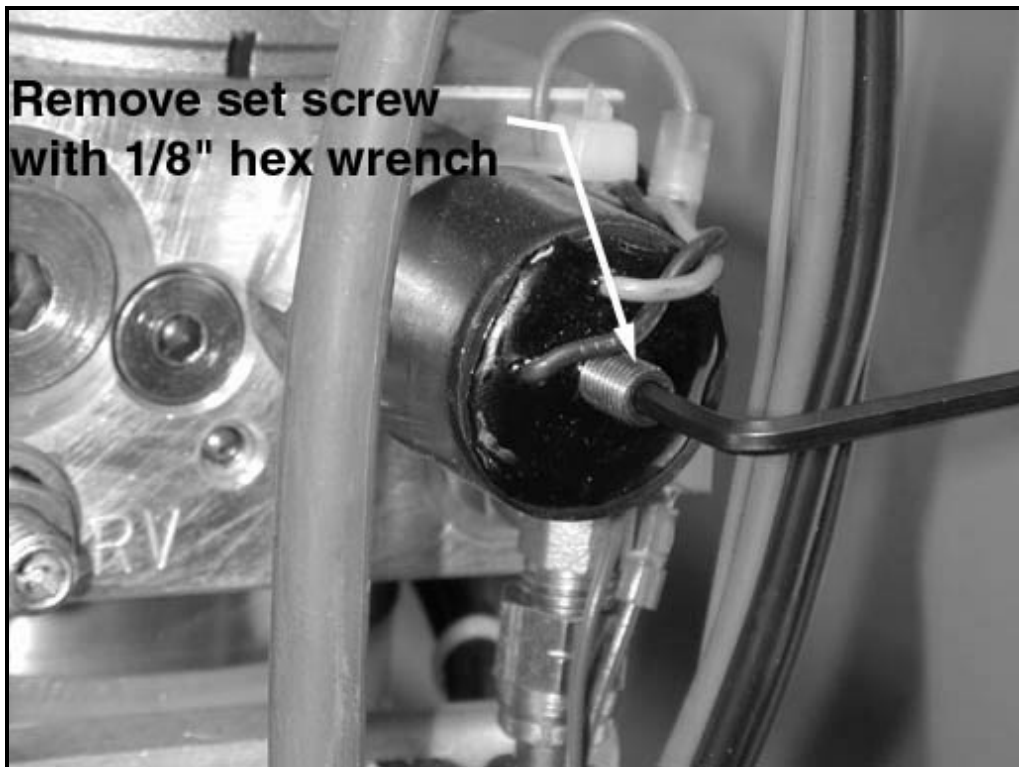
FIG [5]: PRESSURE SWITCH SET SCREW DETAIL
