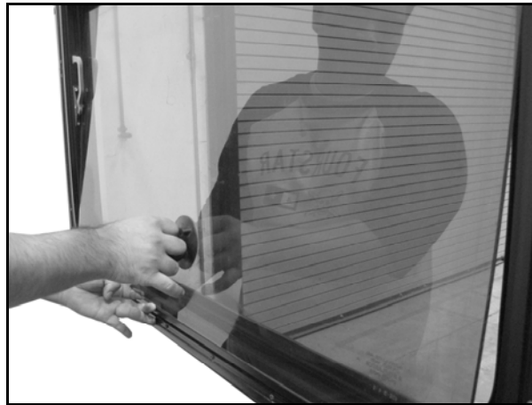
Figure 3-2. PULL STANDARD FRAME WINDOW LINER USING SUCTION CUP
