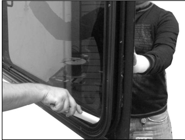
FIGURE 3-18. (EXAMPLE) TWO TECHNICIANS REMOVING HIDDEN FRAME CLIPS
