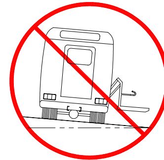
FIGURE 2-1: SLOPED PARKING HAZARD
