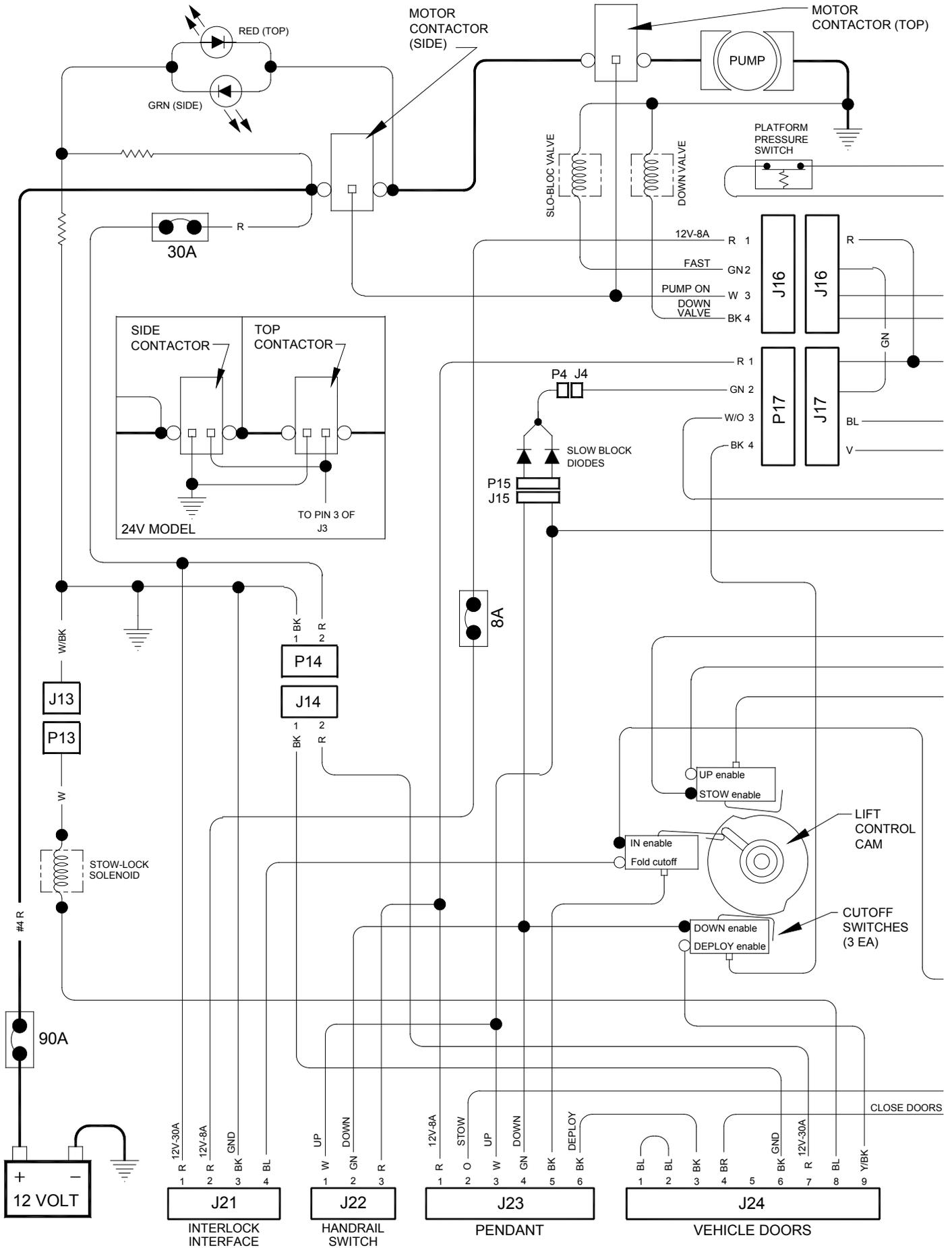
FIGURE 3-9: K-SERIES DOT PRIVATE USE LIFT SCHEMATIC
