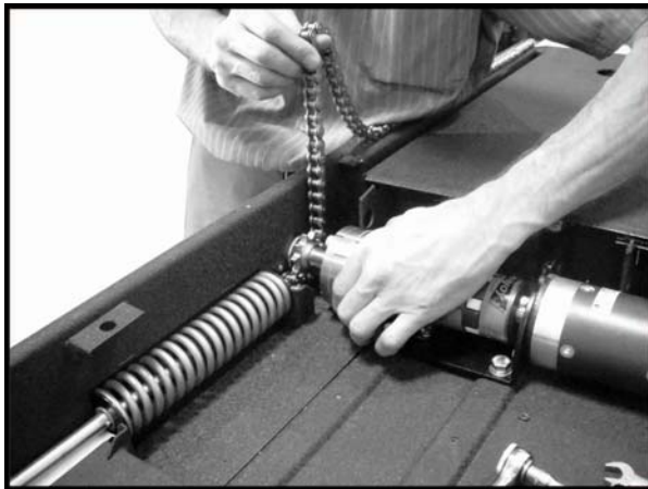
FIGURE 2-7 and 2-8: ROUTE CHAIN SPRING (LH SIDE SHOWN)
