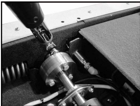
FIGURE 2-18: Torque Each Nut
