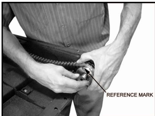
FIGURE 2-12 and 2-13: LARGE SPROCKET ALIGNMENT (LH SIDE SHOWN)
