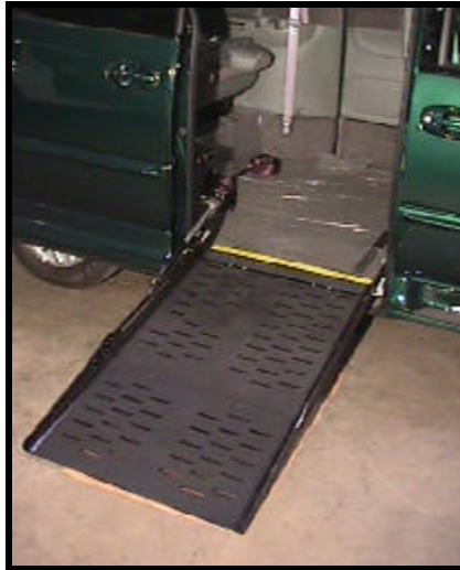
FIGURE [1-2]: FOLDING RAMP DEPLOYED
