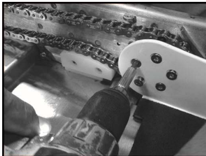
FIGURE 2-20: RAMP TRAY INSTALLATION (RH SIDE SHOWN)
