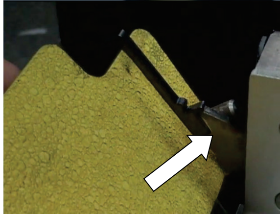
FIGURE 4-16B: ROLLSTOP ADJUSTMENT GAGE TOOL (P/N 55273) IS MATED WITH ROLLSTOP HOOK
