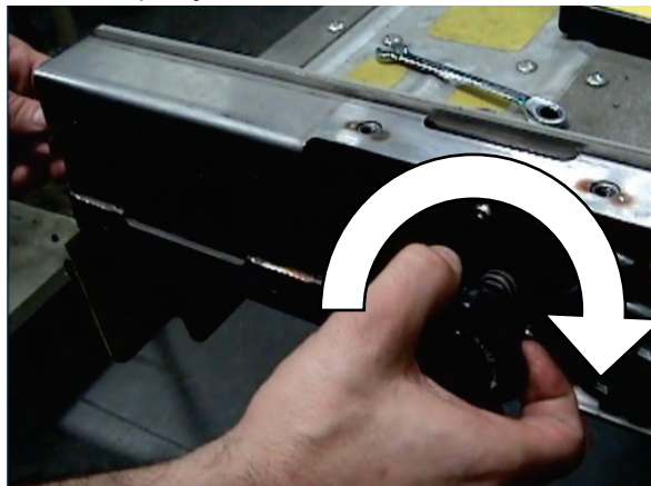
FIGURE 4-15: TURN MANUAL RELEASE KNOB CW TO LOCKED POSITION
