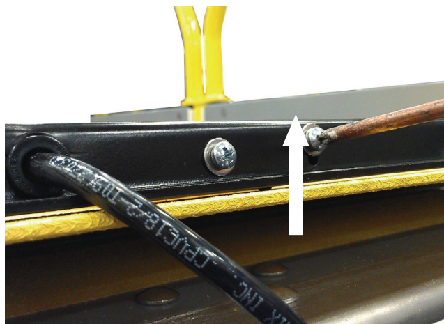
FIGURE 2-12. BRIDGEPLATE SWITCH RESET
