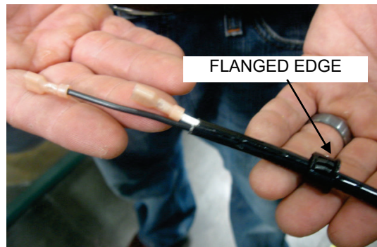
FIGURE 4-28. DISCONNECT BRIDGEPLATE SWITCH CONNECTORS
