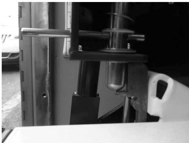
FIGURE 4-42B: VERIFY GAPS WITH TOOL P/N 55273
