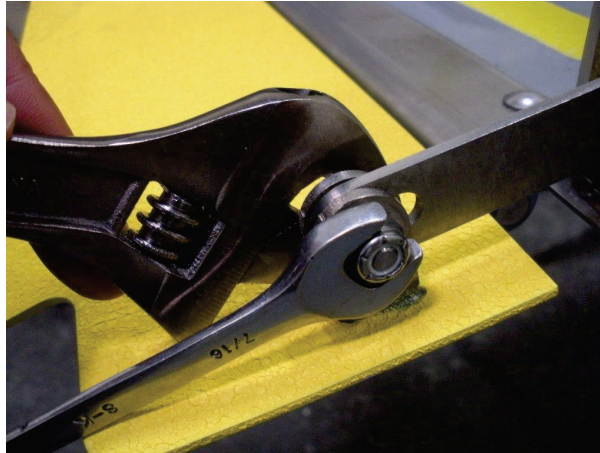
FIGURE 4-14: DETACHING ACTUATING LINKAGE ASSEMBLY FROM ROLLSTOP
