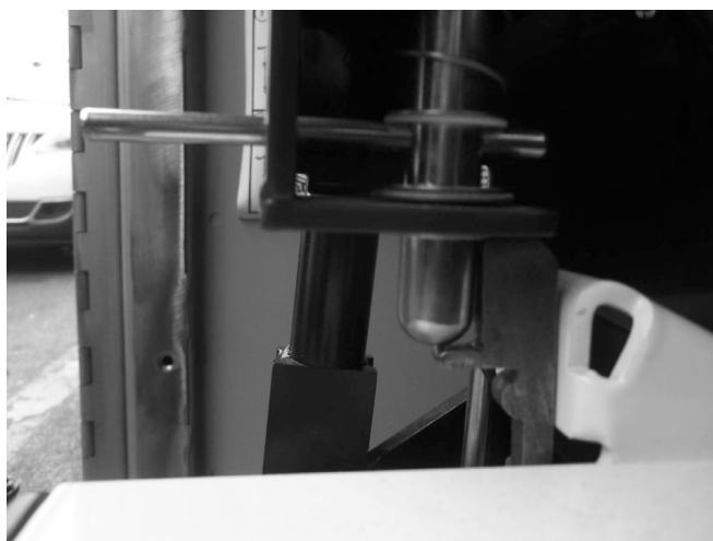
FIGURE 4-42B: VERIFY GAPS WITH TOOL P/N 55273
