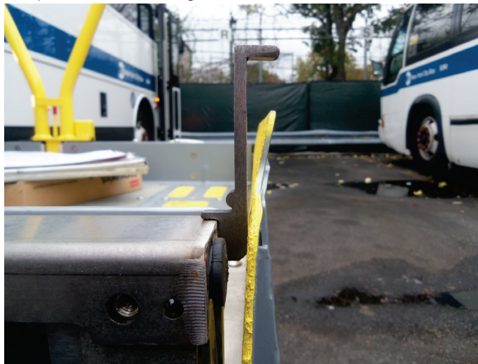
FIGURE 4-18: IN THIS ORIENTATION, GAGE TOOL (P/N 55273) WILL PREVENT LIFT FROM RISING
