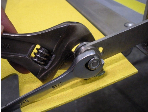
FIGURE 4-14: DETACHING ACTUATING LINKAGE ASSEMBLY FROM ROLLSTOP
