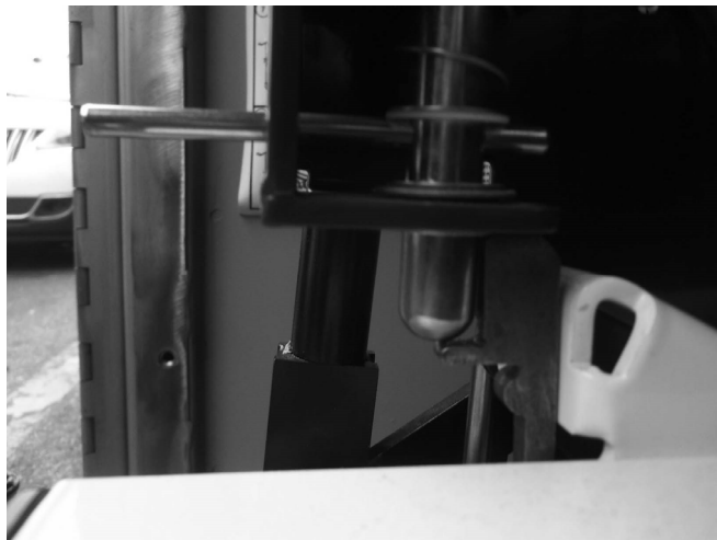
FIGURE 4-42B: VERIFY GAPS WITH TOOL P/N 55273
