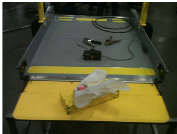
FIGURE 2-7. 25 LB. (11 KG) LOAD TEST (CENTER SIDE)
