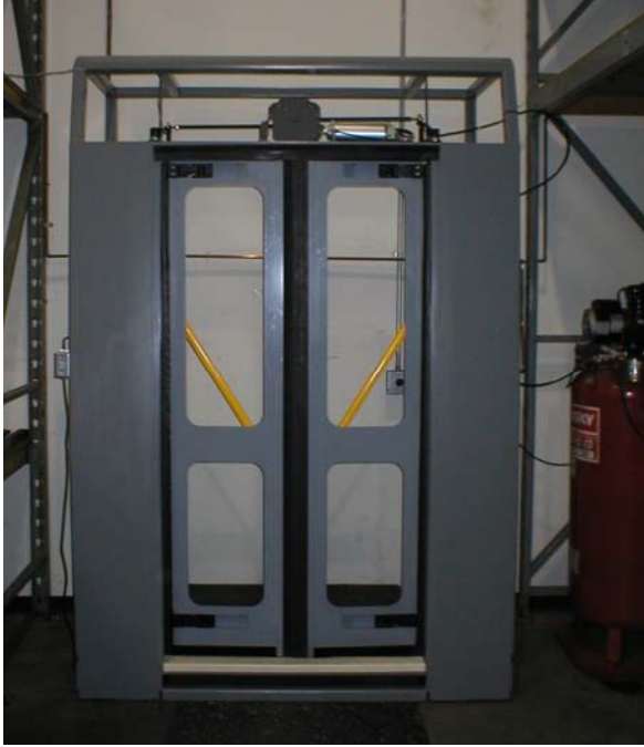
Photo 3: Slide-Glide Door Actuator accelerated lifecycle test (over 500k cycles).
