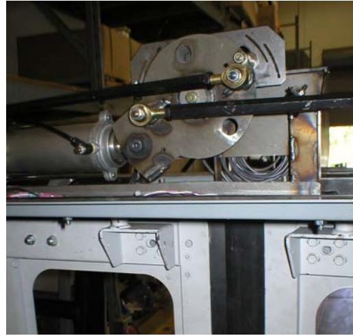
Photo 3: Slide-Glide Door Actuator accelerated lifecycle test (over 500k cycles).
