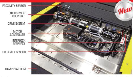
Prime Mover ......24VDC Brushless Permanent Magnet Electric Motor Power Requirements:
