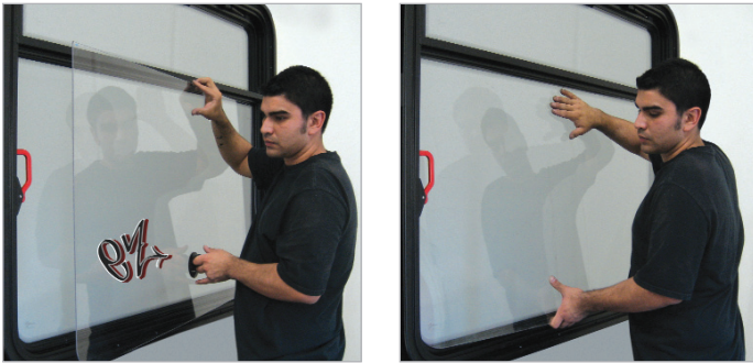
OPTIONAL GLASS GUARD WINDOW LINERS PROVIDE FOR CONVENIENT LINER REPLACEMENT IN LESS THAN 60 SECONDS.
