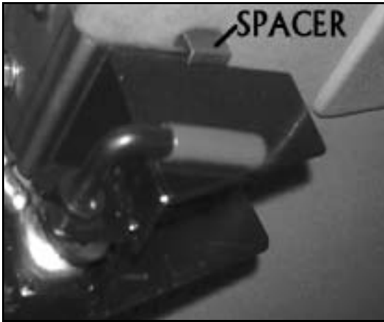
FIGURE [7a]: LEFT-DOOR ANGLE/CLEVIS BRACKET ASSEMBLY INSTALLATION
