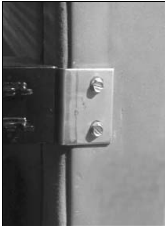
FIGURE [6]: MOUNTED ANGLE/CLEVIS BRACKET ASSEMBLY
