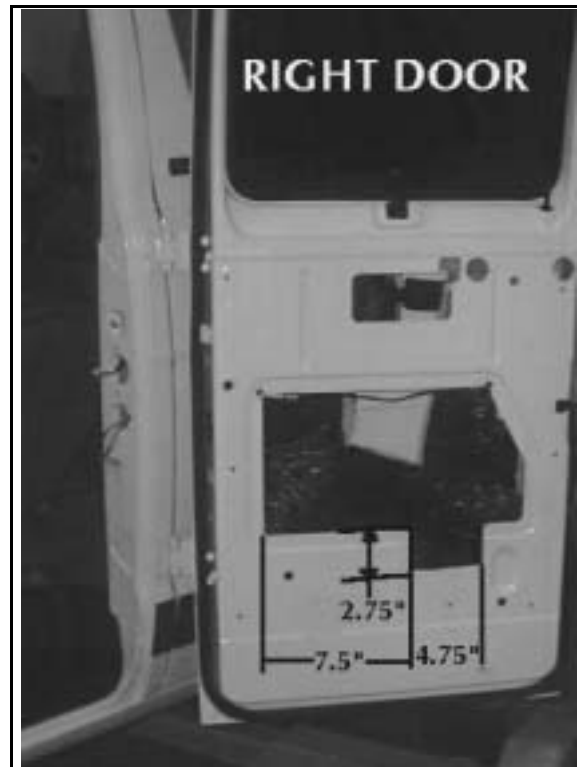
FIGURE [7]: RIGHT DOOR CUT DIMENSIONS
