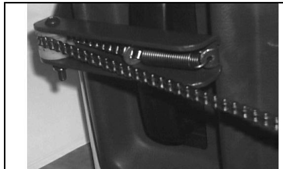
FIGURE [9]: SPRING AND WASHER CONNECTED TO CHAIN
