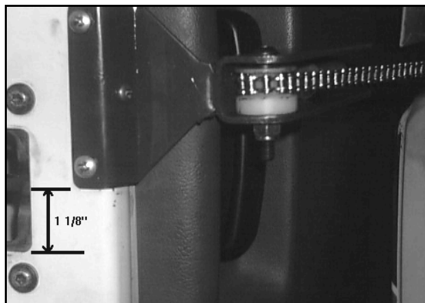
FIGURE [5]: FORWARD DOOR BRACKET INSTALLED
