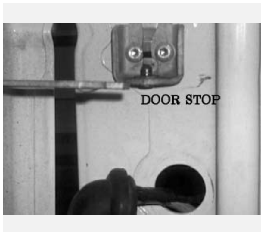
FIGURE [2]: REMOVE ALL DOOR STOPS
