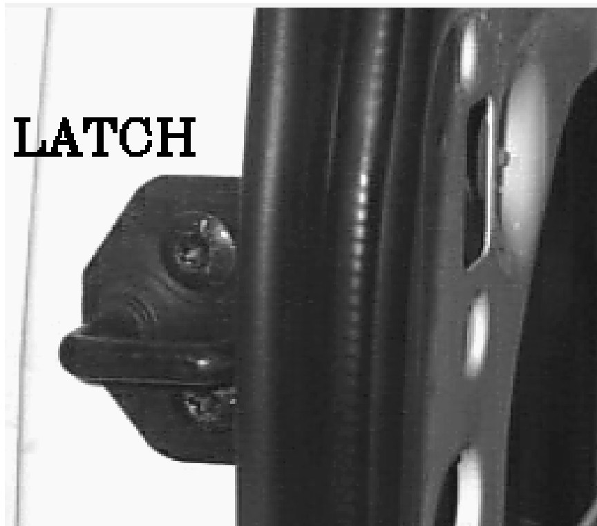
FIGURE [1]: REMOVE ALL LATCHES
