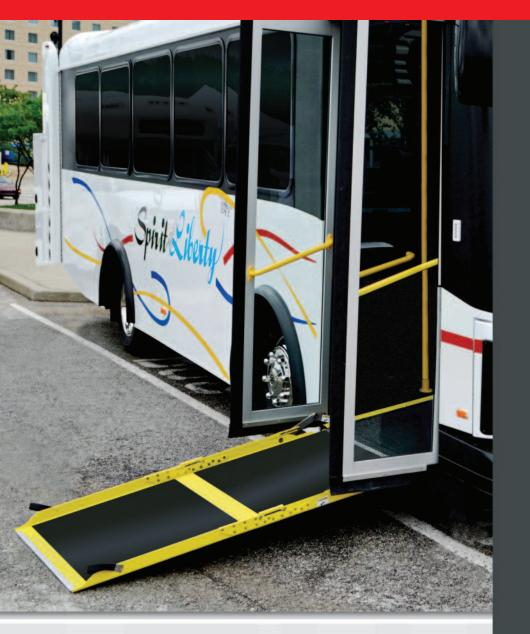
NEW ELECTRIC BIFOLD® BR2E MODEL ACCESS RAMP FOR SMALL, LOW FLOOR BUSES
