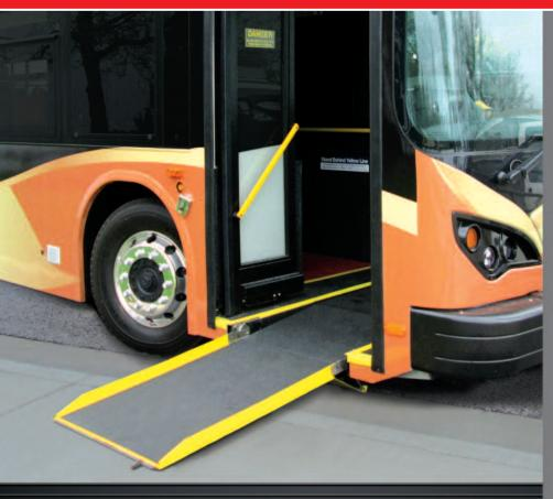
NEW FOLDOVER® 621SA MULTI-SLOPE LOW-FLOOR BUS RAMP WITH OPTIONAL CARBON FIBER PLATFORM
