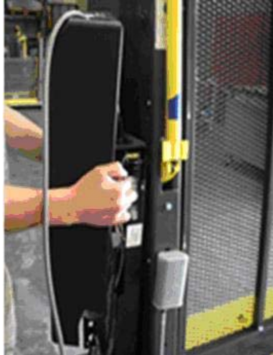
Figure 1. Remove Pump Cover
