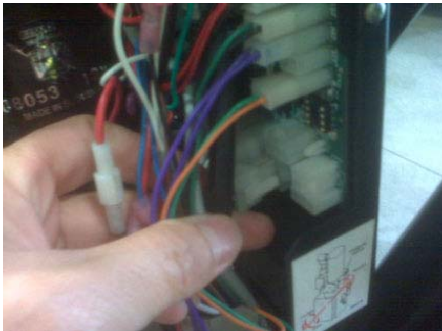
Figure 2. Unplug all PCB Terminals and Receptacles
