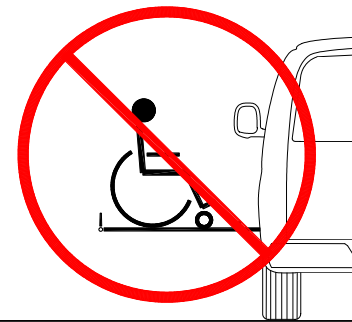
FIGURE 2-2: DON'T EXIT FACING BACKWARDS
