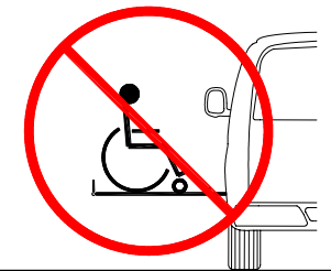
FIGURE 2-2: ALWAYS FACE OUTBOARD WHEN RIDING ON THE LIFT PLATFORM
