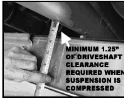
FIGURE 5: DRIVESHAFT CLEARANCE
