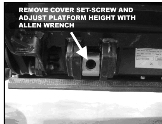
FIGURE 17: ADJUST PLATFORM HEIGHT
