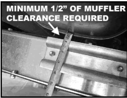
FIGURE 4: MUFFLER CLEARANCE
