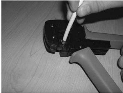
FIGURE 2-7: CRIMPING 8 AWG WIRES
