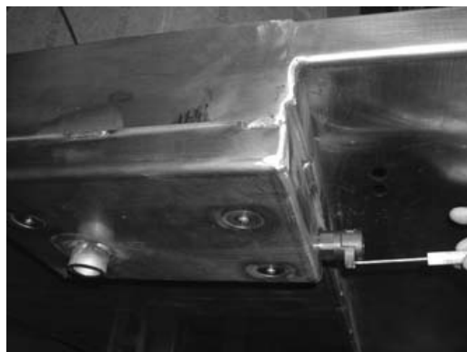
FIGURE 2-6: PASSING WIRE BUNDLE THROUGH HOLE
