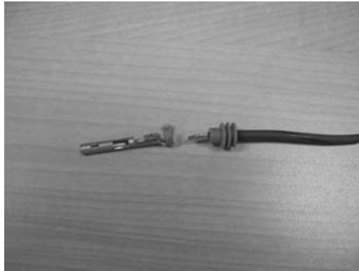
FIGURE 2-8: CRIMPING 14 AWG WIRES
