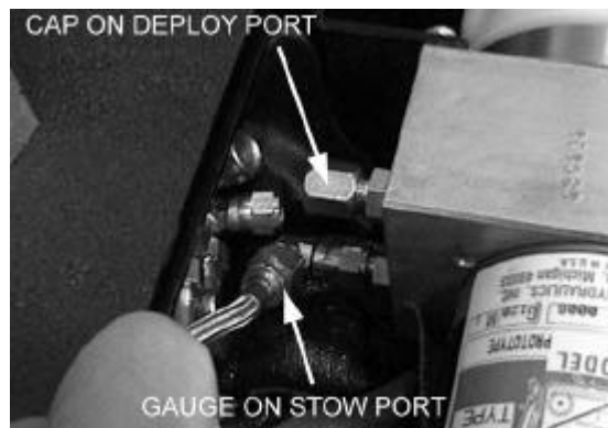
FIGURE 4-2: PRESSURE GAUGE CONNECTED TO STOW PORT
