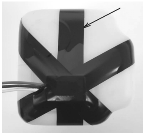
FIGURE 2-3: SECURE SENSOR WITH TAPE WHILE CURING
