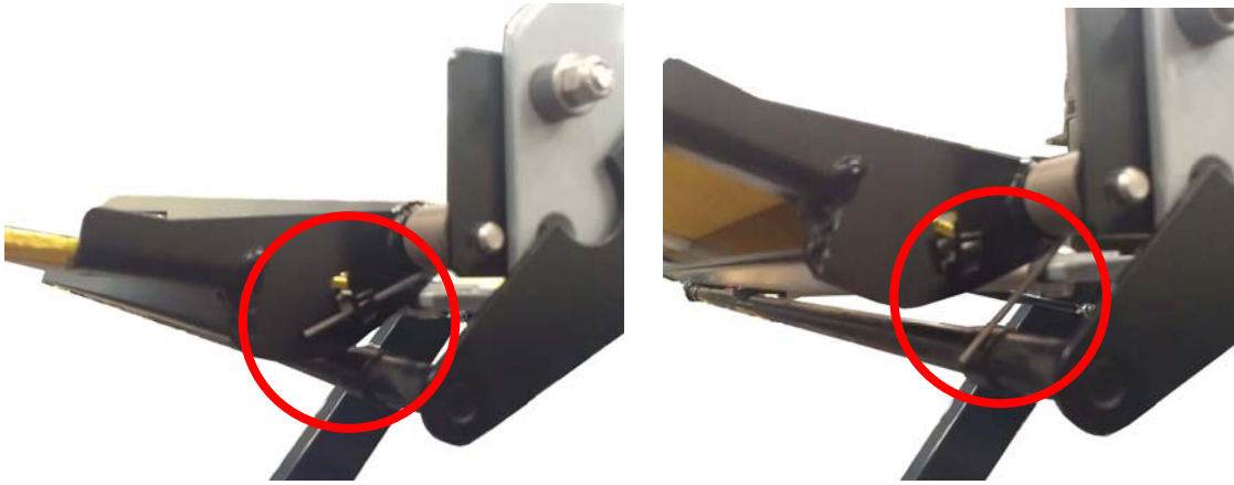
FIGURE 4-25A AND 4-25B. DETACH LH AND RH BRIDGEPLATE TORSION SPRINGS
