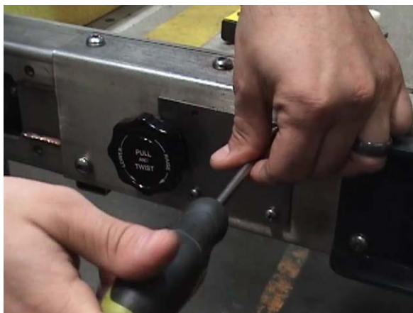
FIGURE 4-9: REMOVE MANUAL RELEASE COVER PLATE AND RH ROLLSTOP COVER
