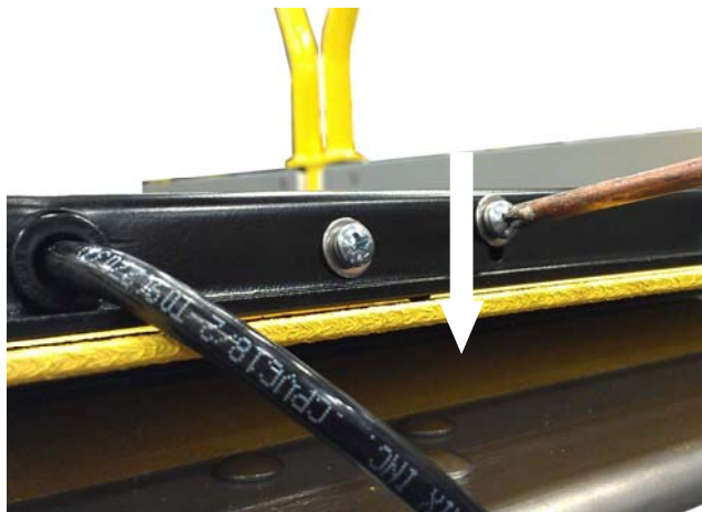
FIGURE 2-14. BRIDGEPLATE SWITCH ADJUSTMENT
