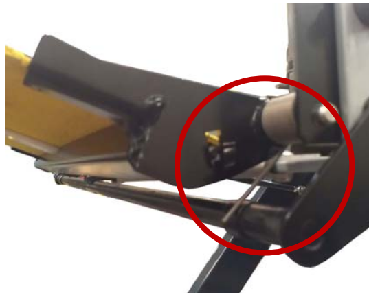
FIGURE 2-10. UNHOOK BRIDGEPLATE SPRING
