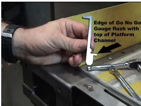
FIGURE 4-5: ROLLSTOP ADJUSTMENT TOOL P/N 55273
