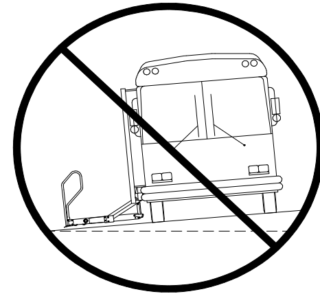
FIGURE 2-1: UNSAFE VEHICLE SLOPING
