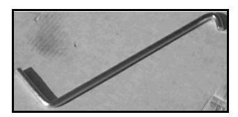
P/N:V2-AC-68 Description: Drift Pin Used W/ Serial Numbers: Below 32000
